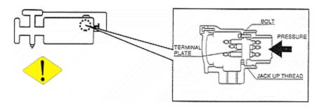
If it is necessary to open the terminal box assembly for any reason, first ensure that mains supply is switched off. Then loose the bolts of terminal box cover by 2 or 3 turns to release internal pressure or liquid if any present in the assembly. You must take all safety measures before opening the terminal box assembly.
