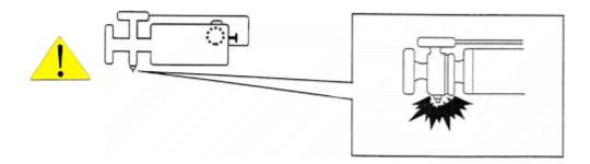
The internal pressure can be higher than the atmosphere. Always loose the drain plug slowly to relieve any internal pressure before attempting to dismantle the pump. You must take adequate precautions, as the liquid in the pump can be hazardous to personnel or the environment.
