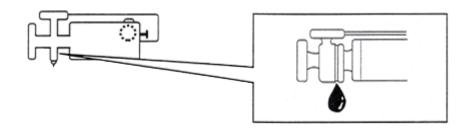
Sudden changes in temperature must be avoided. Rapid changes can cause leakage through gaskets. Published procedures for proper heating and cooling must be followed. If published procedures are not available consult to nearest KIRLOSKAR office before starting the pump.
