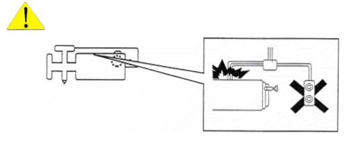
Restarting the motor before finding & rectifying the cause may result in excessive heat generation in the equipment thereby causing pump or motor failure.
