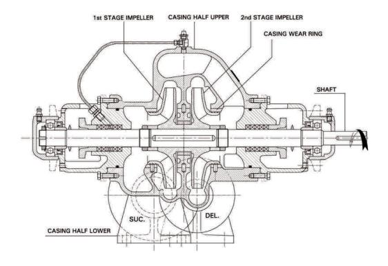
DSM (Non Thru Bore) Pump - Typical Drawing
